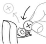
Now place the new battery in the drawer as shown. Close the drawer. If it doesn't close easily, the battery is not placed correctly. If you are not using the hearing aid for a few days, remove the battery.
