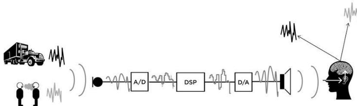
Figure 4. Simultaneously produced speech and noise signals are processed as a single unified signal in the A/D converter. The analysis of the signal into speech and noise components does not take place until after the input signal has been digitized. If the level of the unified signal fed by the microphone to the converter overloads the converter, clipping may eventually result in an inaccurate reproduction of both the speech and noise signals.
