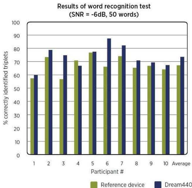
*Figure 3. Results of the speech recognition test. The bars indicate the percentage of correctly identified triplets with the DREAM vs the reference hearing aids.*
