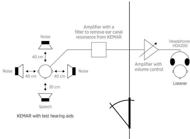
Figure 2. Illustration of the test setup. Speech was delivered from a loudspeaker located directly in front of a KEMAR wearing the test hearing aids, while the noise was delivered via three loudspeakers at 90°, 180°, and 270°. The participants listened to the speech stimuli from an adjoining room through headphones connected to the test hearing aids.
