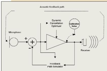
Fig. 6. Diagram of Feedback Cancelling System.
