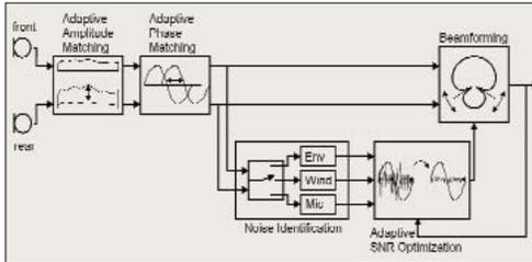
Fig. 5. Block diagram of Locator directional system.
